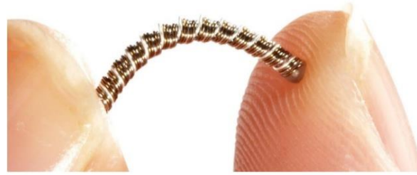
Flexible Ocular Insert for Glucose Measurement
